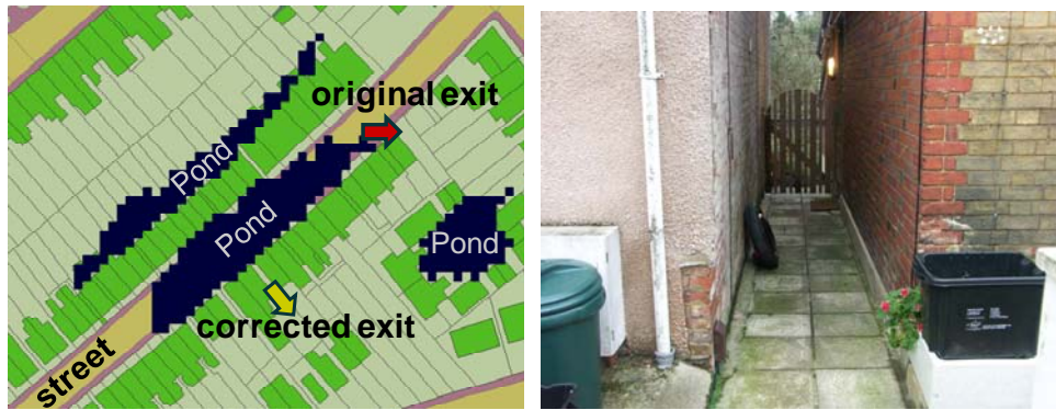
Figure 11. Original pond's exit (upper arrow) was corrected based on the flood reported that flood water escaped at the alleyway between houses (lower arrow).
